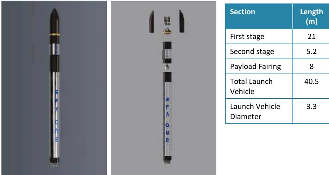
Figure 3.2 RFA ONE NOM Launch Vehicle dimensions
