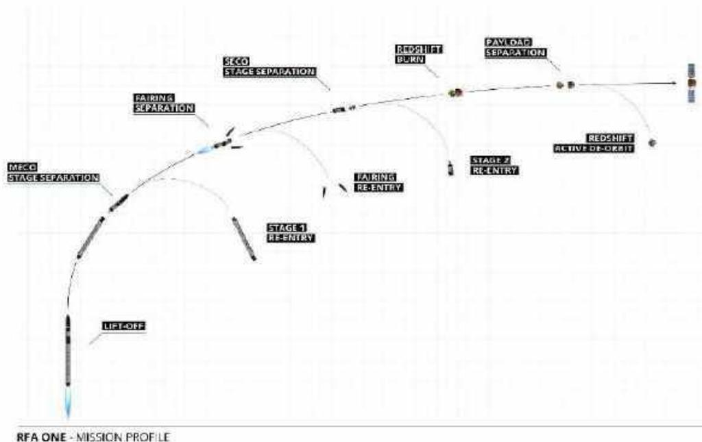
Figure 3.3 RFA ONE NOM typical flight stages
