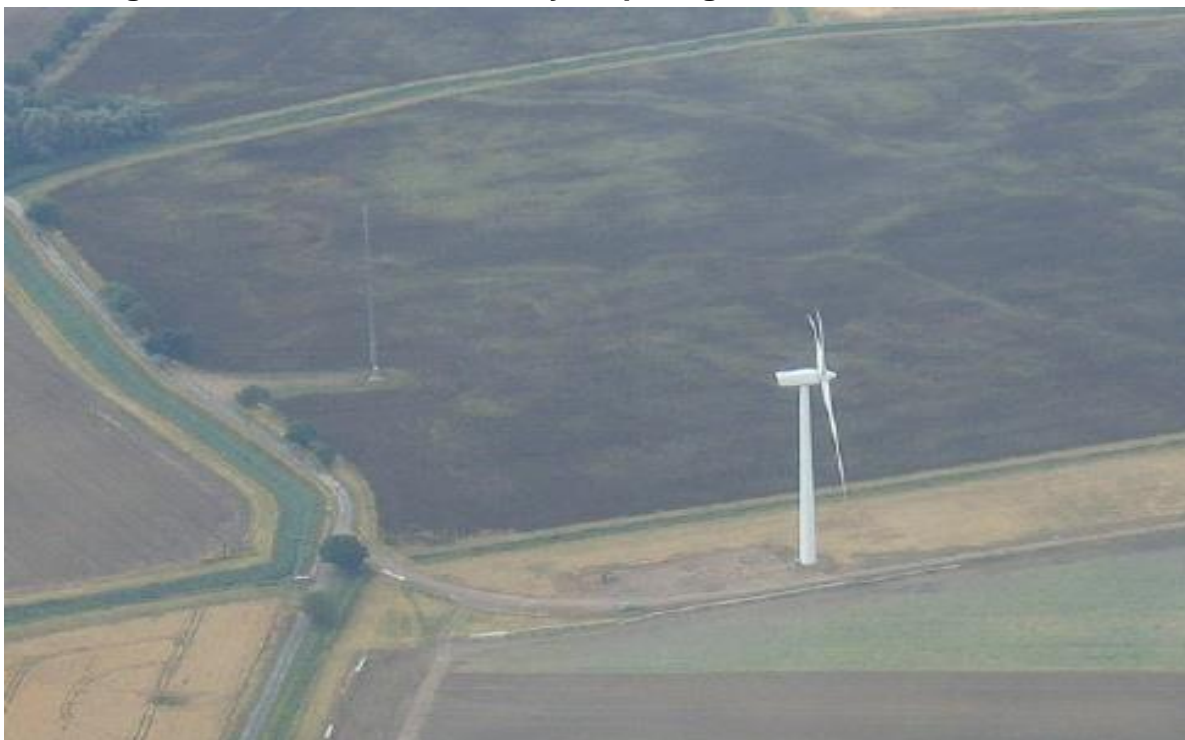
Figure 3: Difficulties in visually acquiring anemometer masts
