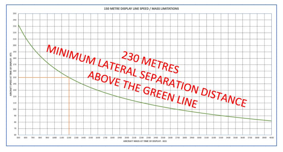
The graph shows a line of constant kinetic energy equivalent to a 1200kg aircraft flying at 150kt. Displays involving combinations of mass and speed under the line may use a lateral separation distance of 150m, subject to FDD agreement. Displays involving combinations of mass and speed that are above the line must use a lateral separation distance of not less than 230m.
