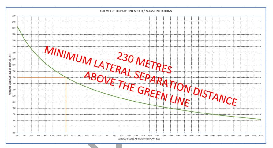
5.41 The graph shows a line of constant kinetic energy equivalent to a 1200kg aircraft flying at 150kt. Displays involving combinations of mass and speed under the line **may** use a lateral separation distance of 150m, subject to FDD agreement. Displays involving combinations of mass and speed that are above the line **must** use a lateral separation distance of not less than 230m.
