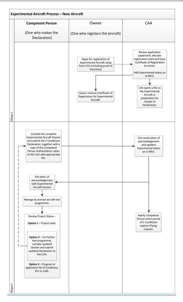
This flowchart shows the process of starting an E Conditions project with a new aircraft design. It is a visual summery of the E Conditions process outlines in the CAP.
