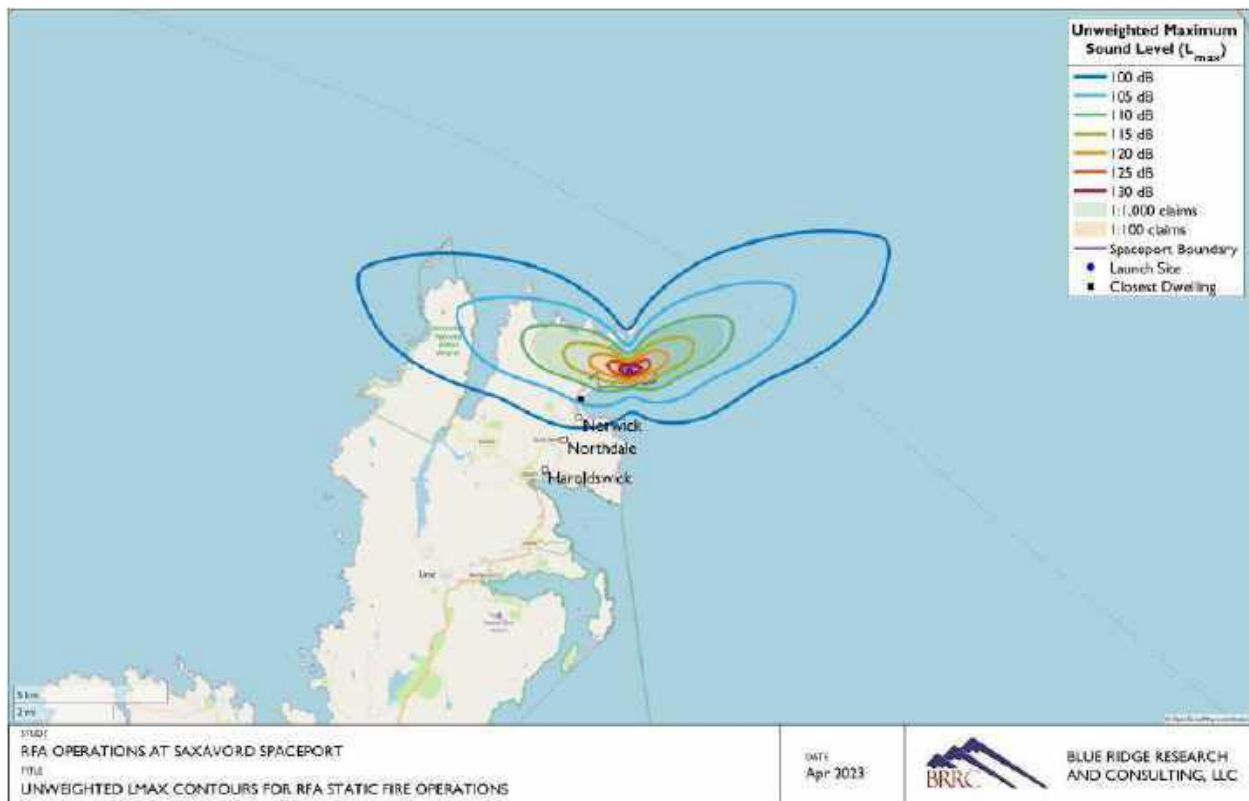
Figure 6. Unweighted maximum sound level contours for RFA ONE static fire operations.
